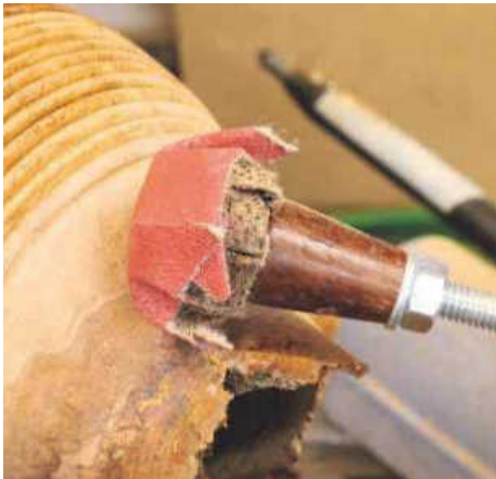
STEP 23. This little hook-and-loop sanding ball is fantastic for sanding the inside. The abrasive needs to be cut like a flower petal and then just wrapped around the ball
